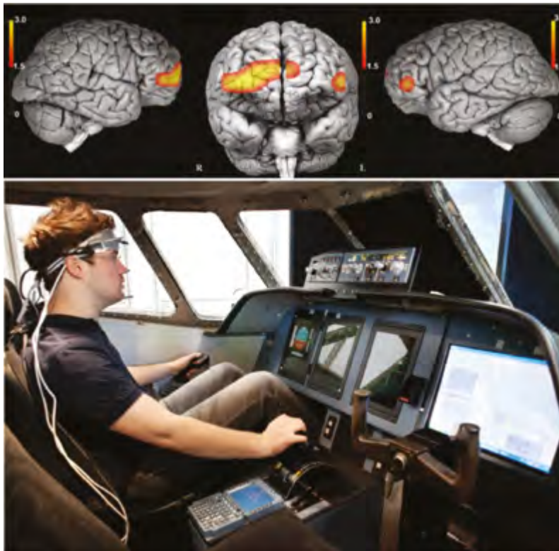
A simulator hooked up to a near infrared spectroscopic imaging device. Frédéric Dehais, CC BY.
